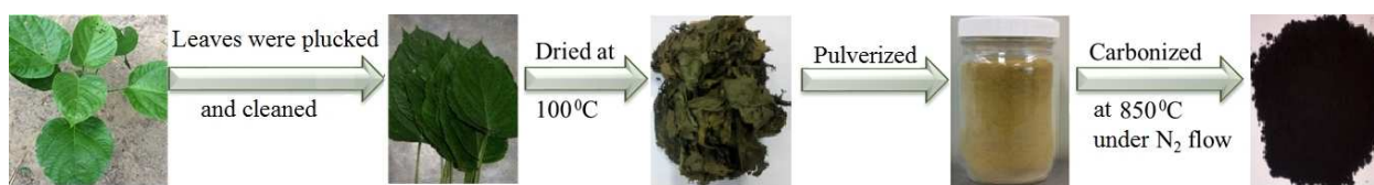
Scheme 1. Schematic representation of the preparation of NDC from Bhand leaves.
