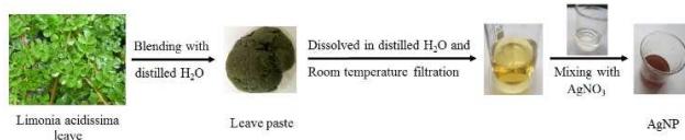
Scheme 1. Schematic illustration of AgNP synthesis from Limonia acidissima leaf extract at room temperature.
