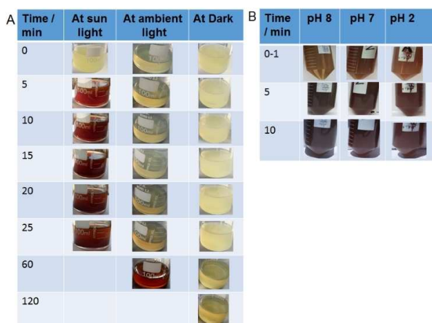
Figure 3. A) Effect of time and light on AgNPs synthesized by the reaction of leaf extract (0.25 g/mL) with 0.0027 M \text{AgNO}_3 and B) effect of pH under sunlight.
